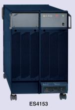
The ES4152 and ES4153 Reference Impedance Networks use a network of resistance and inductance circuits to approximate the impedance of an actual commercial line from the output impedance of the ES series. They are used in combination with the ES series for flicker measurement and harmonic current measurement (JIS standard).
