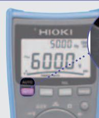
The display freezes automatically when the measurement value is stable.
