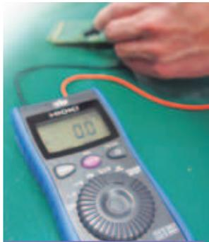
**Test leads plug into the rear**
