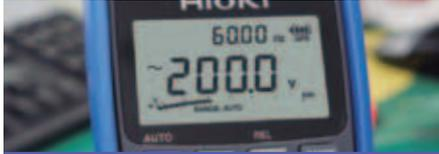
Bar graph refreshes 40 times/second. Acts just like an analog meter to intuitively expose changes in the measured signal.
