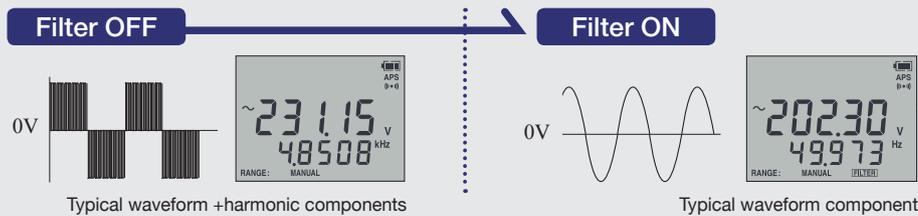
For inverter secondary output voltage measurements, harmonic contents are cut so that the fundamental waveform can be measured.
