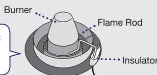
Select the 600.00  $\mu$ A DC range for burner flame current measurement.
