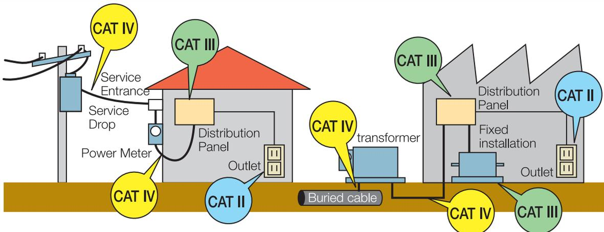
Higher-numbered categories correspond to electrical environments with greater momentary energy, so a measurement product designed for CAT III environments can endure greater momentary energy than one designed for CAT II .
