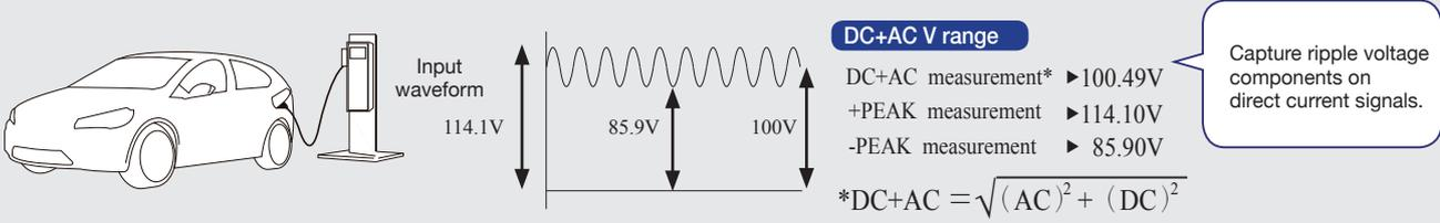
Capture ripple voltage components on direct current signals.
