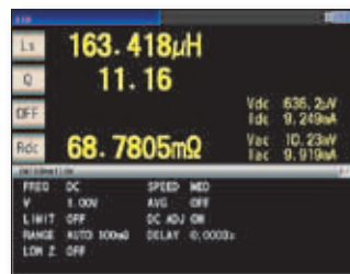
L/Q (1 kHz, 1 mA constant current measurement) and DCR (DC measurement) display screen
