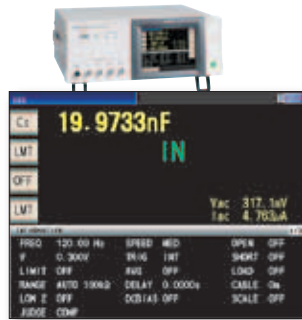
LCR mode Cs display screen (1 kHz measurement)
