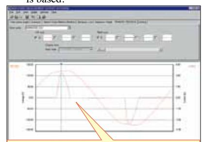
View the waveforms to confirm distortion conditions
