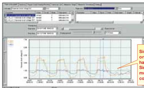
Simultaneously display multiple orders to confirm changes in harmonics!
