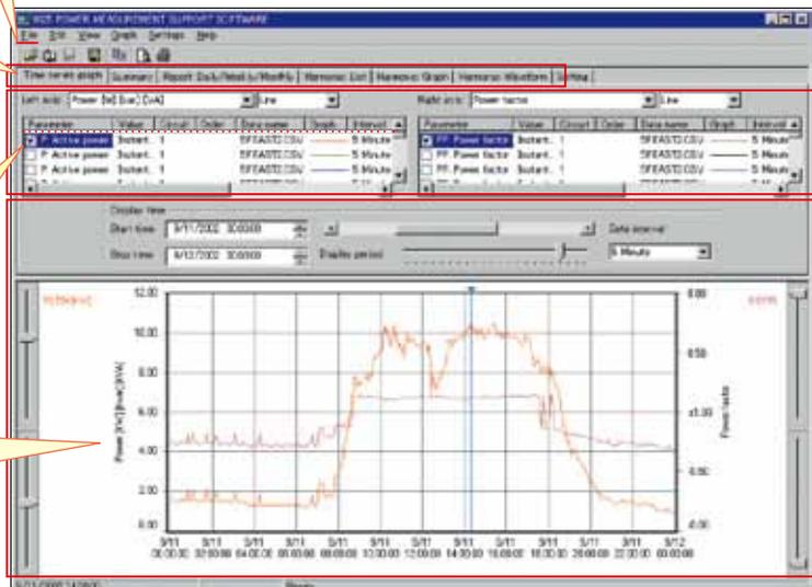
**Time Series Graph Display Function** (two-axes display possible)
