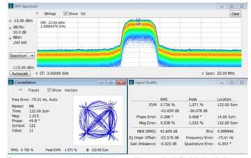
Time-correlated views in multiple domains provide a new level of insight into design problems not possible with conventional analyzers. Here, modulation quality and the constellation measurements are combined with the continuous monitoring of the DPX \*spectrum display.
